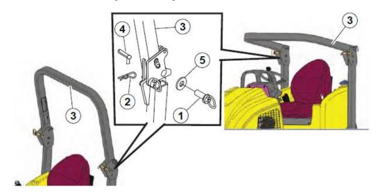
1. Support the upper half of the ROPS (3) using a crane and suitable rigging capable of supporting 19 kg.
