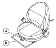
**Note:** Do not change position of the operator's seat while the machine is moving. The "OPERATOR PRESENCE" safety device will prevent all machine movements if an operator is not seated.
