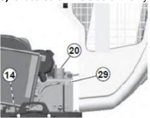
While the machine is turned off, check that the hydraulic oil level is visible at the middle level or higher in the sightglass. If it is not, add oil through the filler port **(20)** inside the engine compartment. Use only clean hydraulic oil.
