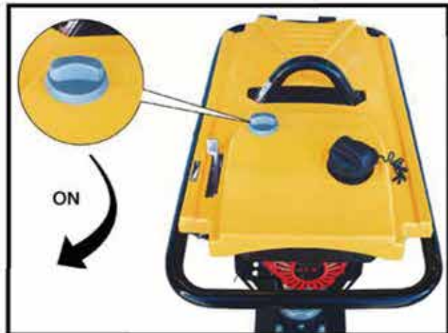
2. On the top of the rammer, turn the fuel switch to the "ON" position
