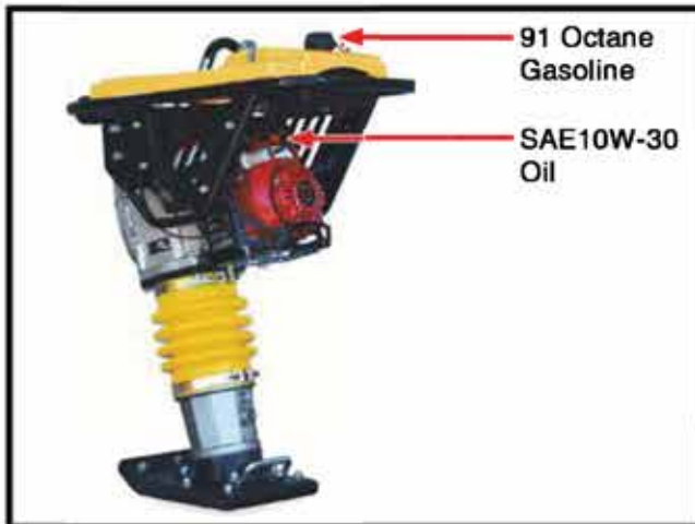
1. Add oil & gas to the rammer's engine
