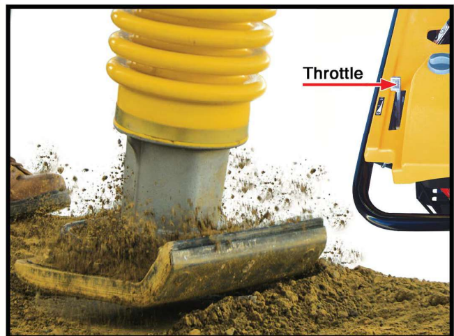
4. Let the engine idle at 1/4 load for 1 minute. To run the machine, move the throttle forward.
