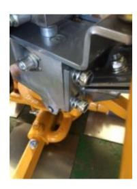
3. Turn the Blade Pitch Handle counter-clockwise.
