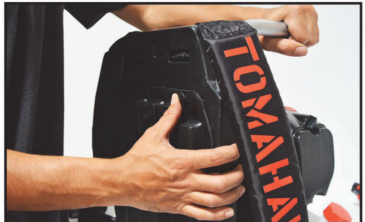
30 Snap the padding brackets back into place
