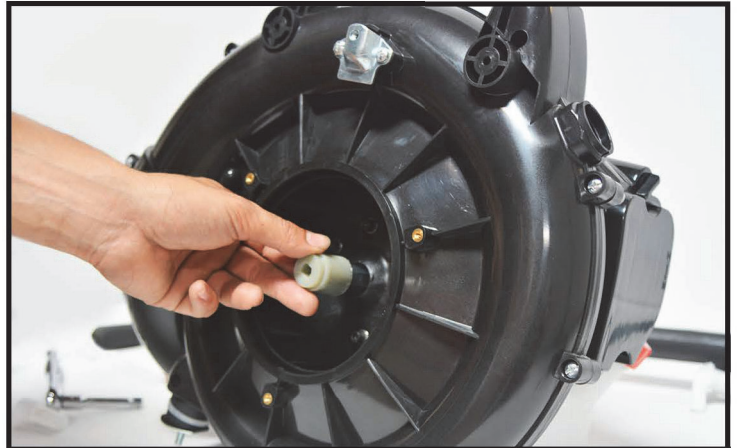
22 Place the plastic coupling onto the aluminum shaft
