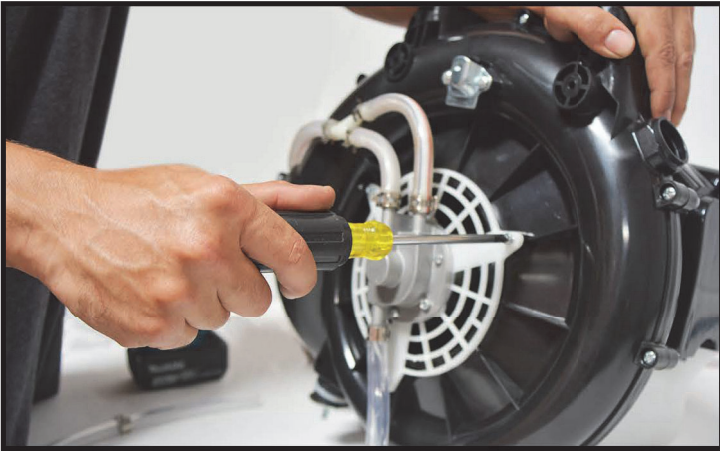
25 Fasten the booster pump to the blower housing
