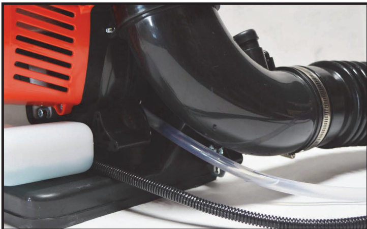
39 Locate the longer booster pump tube near the base of the unit
