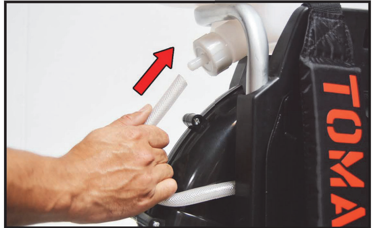
38 Attach the shorter tube from the turbo boost to the base of the chemical tank
