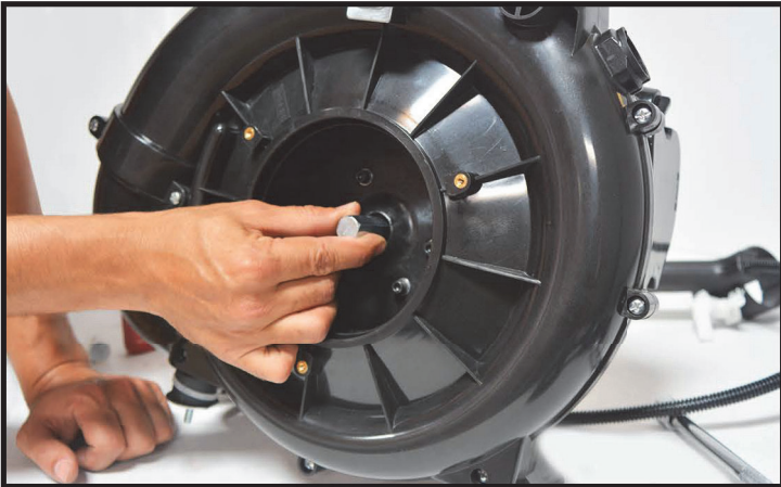
19 Place the aluminum shaft in the back of the blower housing
