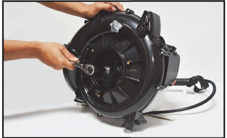
20 Tighten the aluminum shaft
