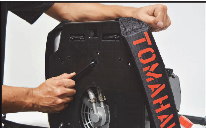
29 Tighten the bolt with an allen wrench
