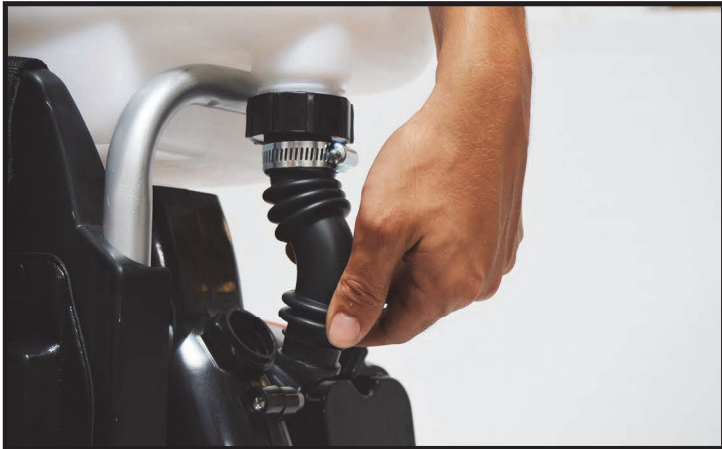
37 Reattach the black tube to the blower housing
