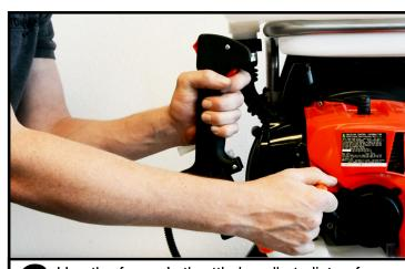
Use the fogger's throttle handle to listen for a high pitch, steady hum & find the right speed
