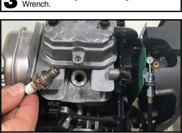
Test the plug by touching it to the metal cylinder & pull the recoil starter several times.
