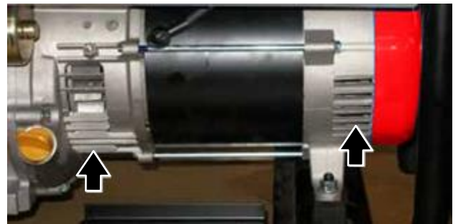
Figure 46 – Alternator Cooling Air Inlet and Outlet Port
