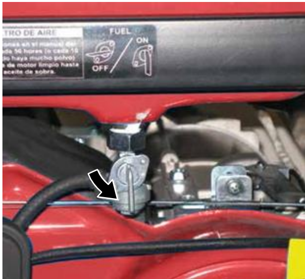
Figure 22 – Fuel Shutoff Valve in the ON Position
