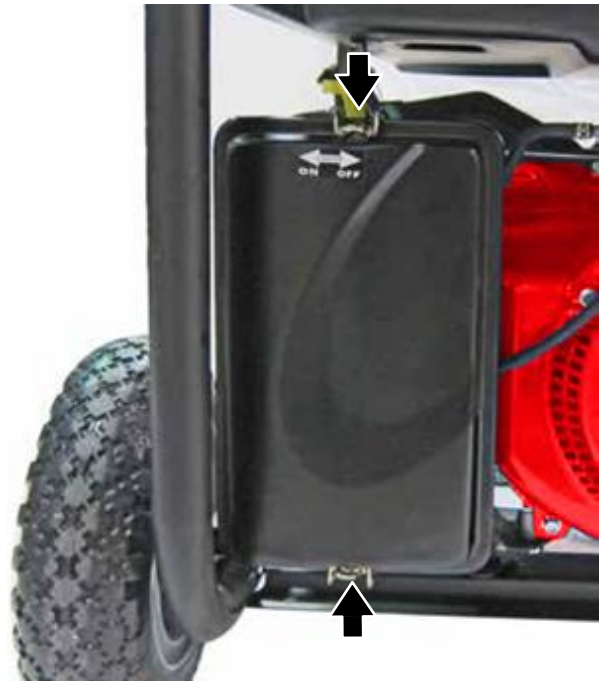
Figure 35 – Installation of Air Filter Cover
