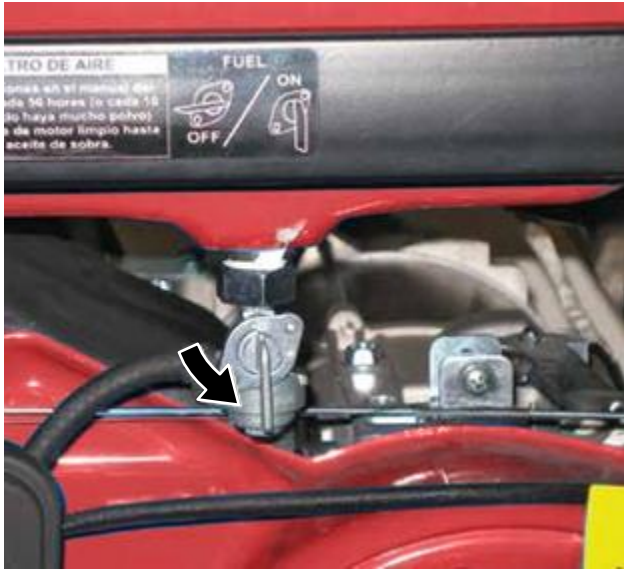
Figure 17 – Fuel Shutoff Valve in the ON Position
