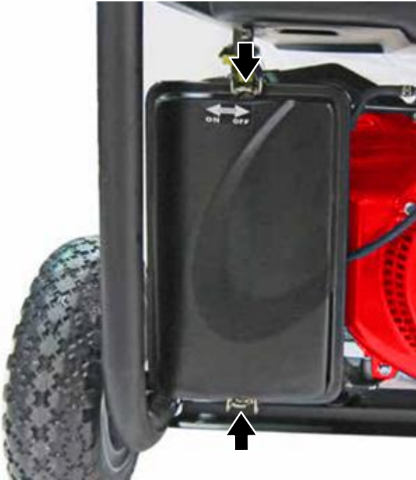
Figure 30 – Removing Air Filter Cover
