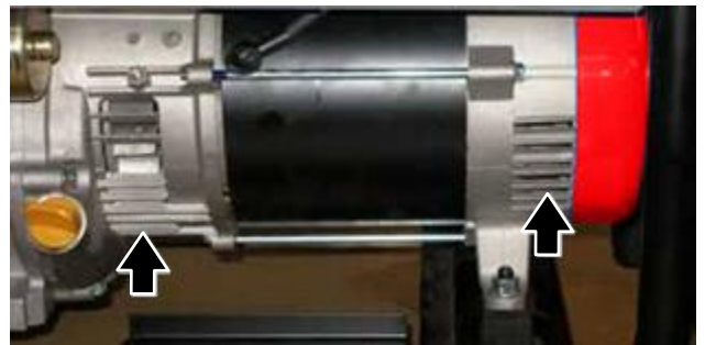
Figure 46 – Alternator Cooling Air Inlet and Outlet Port
