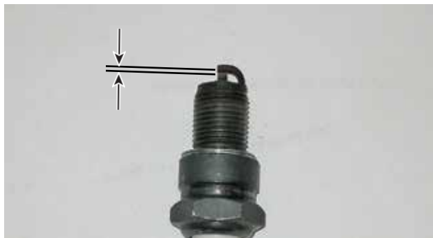
Figure 38 – Spark Plug Gap Requirements
