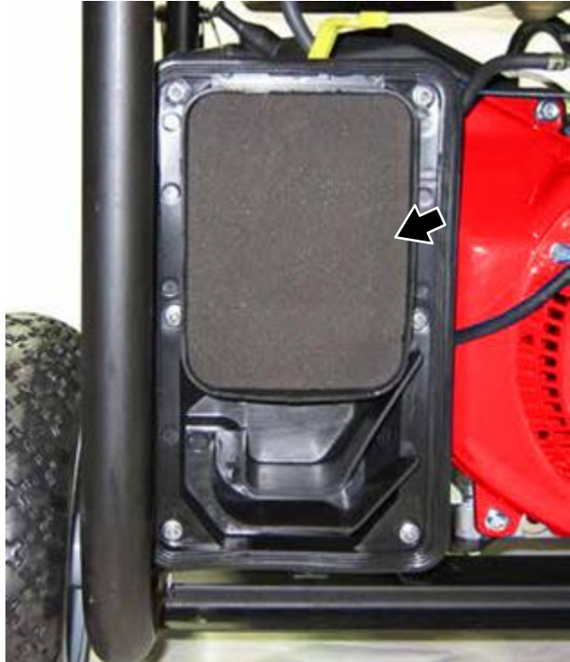
Figure 32 – Removing Fine Inside Air Filter
