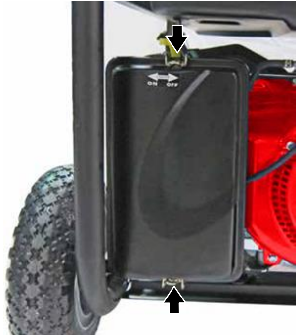
Figure 35 – Installation of Air Filter Cover
