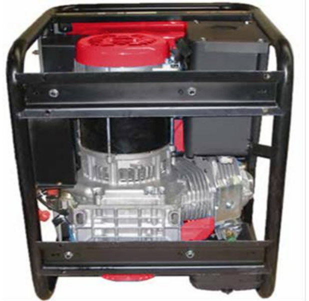
Figure 4 – Tip the Generator onto its Side
