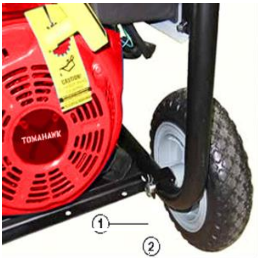
Figure 6 – Assemble Wheels to Frame
