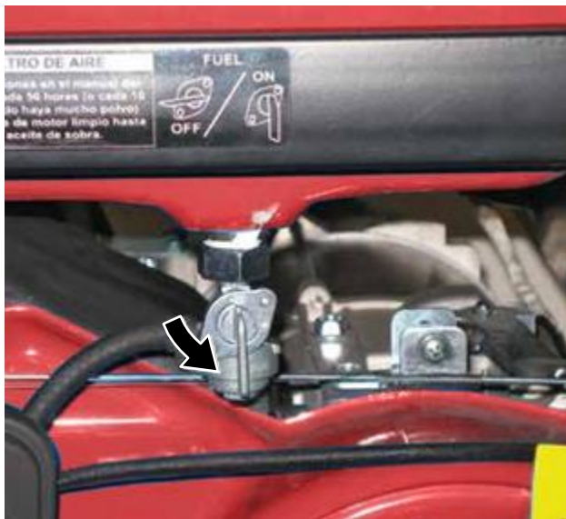
Figure 22 – Fuel Shutoff Valve in the ON Position
