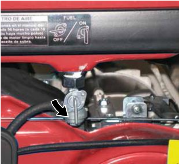
Figure 17 – Fuel Shutoff Valve in the ON Position
