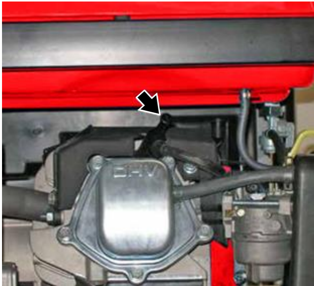
Figure 36 – Removal of Spark Plug Boot
