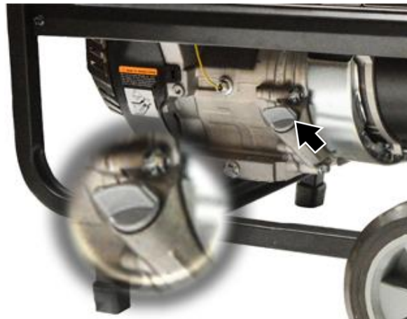
Figure 26 – Oil Fill Plug/Dipstick
