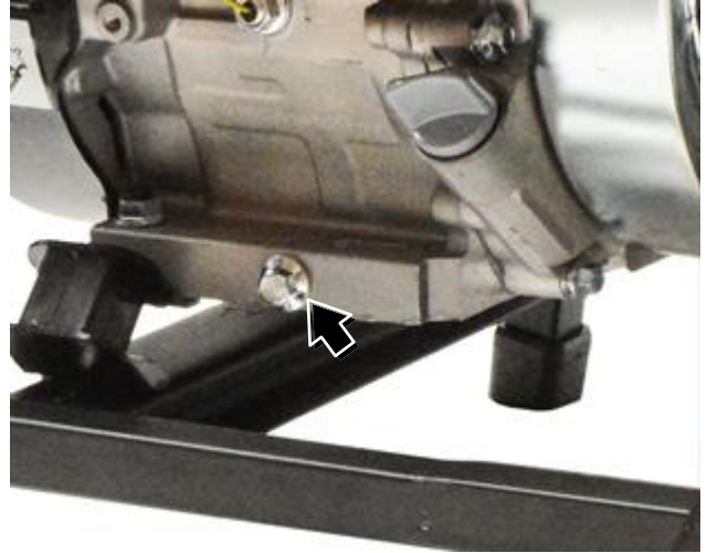
Figure 29 – Oil Drain Plug
