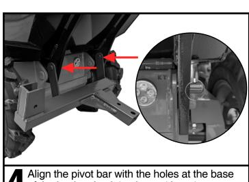
of the bucket. Lock in place with a pin.
