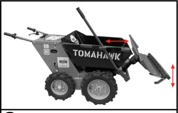
The snow plow can be raised and lowered using the plow handle.
