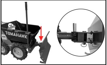
Place the pivot pin in the pivot bar and secure in place with the lynch pin.
