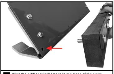
Align the rubber guard's bolts to the base of the snow plow. Tighten with a 13mm wrench and 13mm socket.
