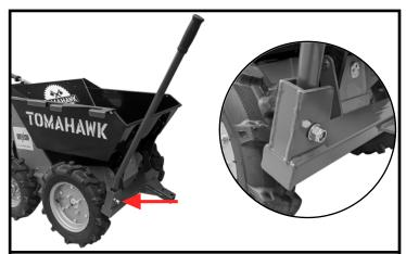
Secure the plow handle in place with the bolt, washer, and nut-tighten with a 19mm wrench and adjustable wrench.
