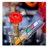
ADJUSTABLE PRESSURE Adjustable from 50 - 500 PSI for even spraying with a aluminum, copper, and brass pump!
