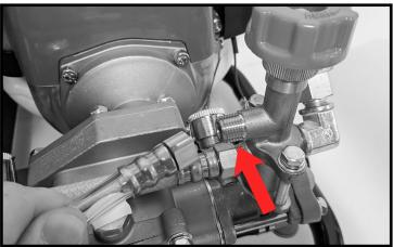
Attach the end of the clear tube below the pressure adjustment knob.
