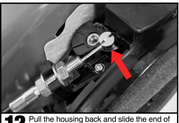
the cable into the engine's throttle terminal."
