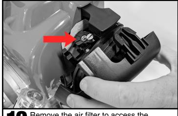
Remove the air filter to access the engine's throttle control terminal.
