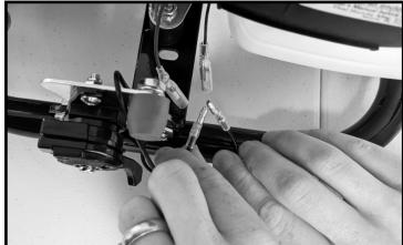
Connect the throttle wires to the Honda Engine wires. Left to Left. Right to Right.
