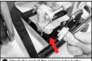
Attach the end of the orange tube to the base of the pump.
