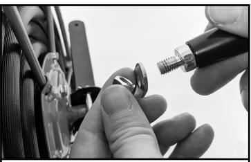
Attach the reel handle using the nut included in the packaging.
