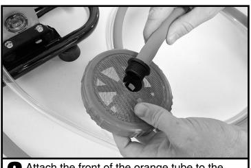
Attach the front of the orange tube to the filter.
