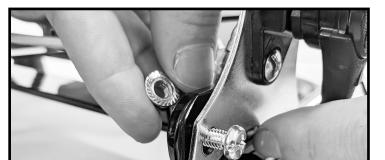
Attach the throttle control using the last 2 screws and nuts.
