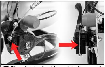
Place the throttle cable end into the gap and fit the cable along the top of the throttle.
