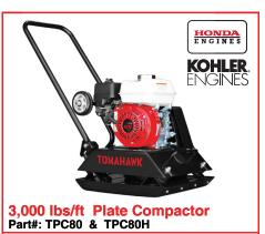
6 HP Kohler CH260 & 5.5 HP Honda GX160 Engines Easily achieve a 100% compaction rating 16.5" x 21.5" plate for narrow trenches and corners Optional Honda Engine model: TPC80H 3 Year Engine Warranty & 1 Year Product Warranty
