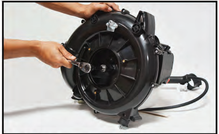
20 Tighten the aluminum shaft
