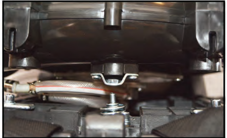
28 Reattach the back plate using the bolt and washer
