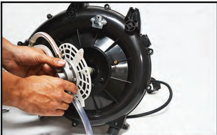
23 Fit the booster pump onto the plastic coupling
