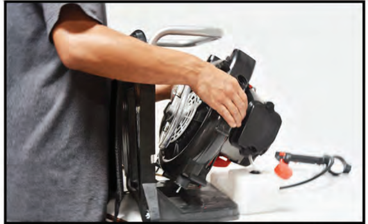
26 Place the blower housing back on the back and base
