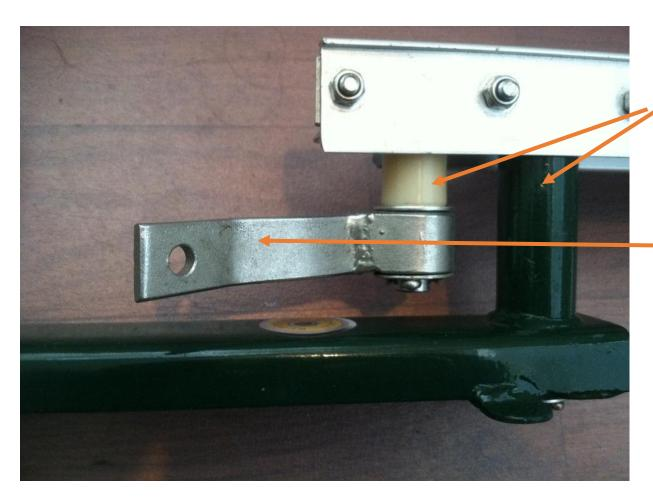
Lubricating both pivots very well, usually resolves the issue and allows the arm to release.
