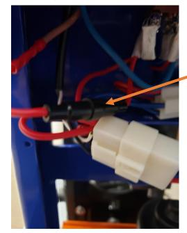
Inline Fuse located here. (This is under the main frame toward the back of the machine)
