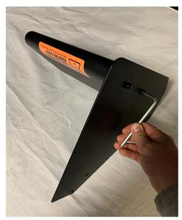
3. Place the back piece onto the frame and using the remaining 6MM allen screws, tighten the back into place with the label to the outside. Make sure the hanging rod has been installed prior to tightening.
