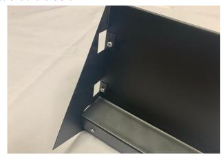
2. Attach the first side wall using three phillips screws through the back then two through the bottom of base into the tabs on side wall. Make sure the tabs go underneath the base. Do not fully tighten screws until the end.
