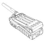
Slide down the battery for about 1 centimetre, and then remove the battery from the radio's body.
