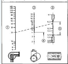
Example: A pipe with Ø 8 x 1 mm (NW 6) is required for a volume of 20 l/h and an average flow rate of approx. 0.23 m/s.
