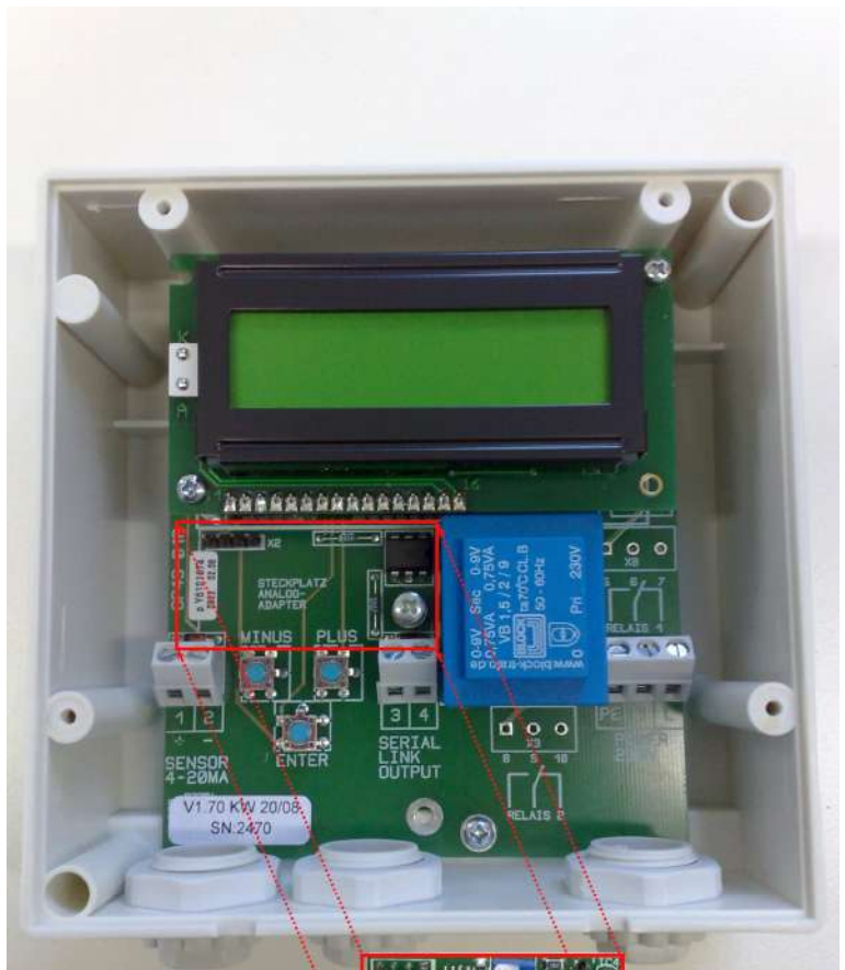
Plug the adaptor onto the contact strip and fasten it with an M3 screw.
