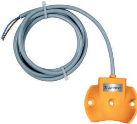
The floor water probe "BWS 10-1" is simply placed on or fixed to the lowest point of the floor surface to be monitored. It detects conductive liquids starting at a level of 2 to 3 mm. The floor water probe has two stainless steel electrodes; it is fitted with a two-wire signal cable.
