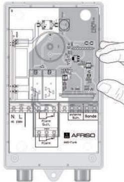
3. Push the antenna of the EnOcean® wireless module into the three housing openings of the product.
