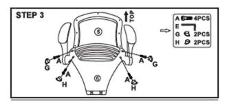
Leave all 4 bolts loose when assembling the arm piece to the back. Start on the lower left. Once that bolt is started, move to the lower right, then the two top bolts. Completely tighten once all bolts have been inserted.
