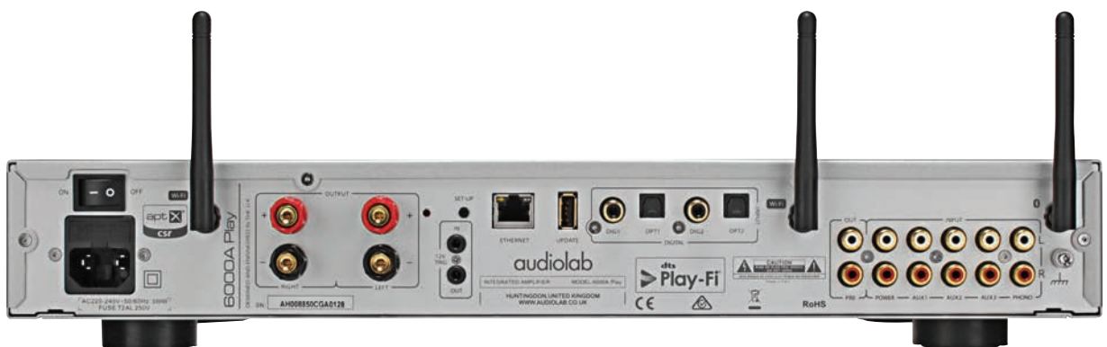
Twin wi-fi aerials (left) and a Bluetooth aerial (right) ensure good radio reception at long range. Crucial to wi-fi connectivity was a tiny activation button beside the central RJ45 ethernet connector (centre). The Digital 1 and Digital 2 inputs (centre right) differed in that the latter can have Wide digital capture applied – an unusual function.
