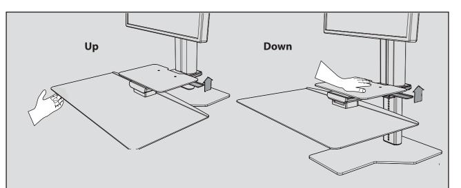
To raise the keyboard and monitor, pull the actuator handle (located under the work surface) upwards to release the lock. If additional force is required, apply a slight upward force to the opposite corner of the work surface or keyboard tray.
