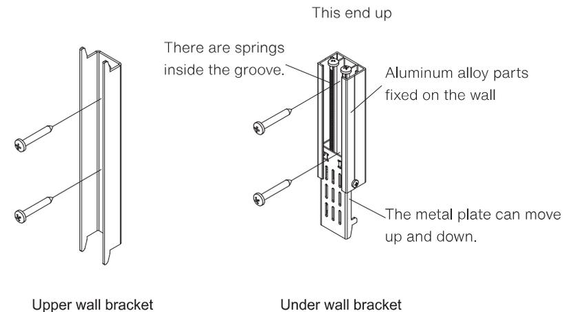
6.2 Install wall hangers on the wall according to screen size. Required tools: level, hammer drill, pencil, ladder, etc. As shown below, the horizontal direction is about 30cm away from both sides of the screen. Please estimate the installation position of the screen before installing the wall pendants. The height of the lower edge of the screen from the ground is generally about 600~800mm.
