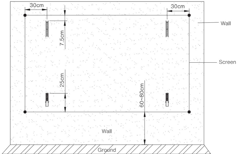
6.3 Hang the screen on the wall according to the method shown in the picture.
