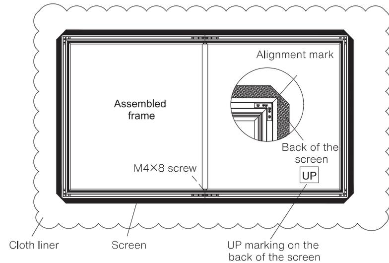
4.4 Hook the screen on the frame with a tension spring. To hook the tension spring, please follow the following sequence, first, hook 1~8 springs; then hook springs 9~12, and then hook other springs from the middle spring to both sides in turn. Please refer to the attached drawing for the installation method of the tension spring.
