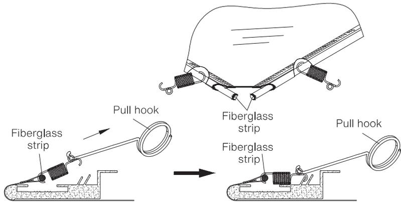
4.5 After hanging the spring, stand the screen up and check the overall flatness of the screen. If there is unevenness, the spring needs to be adjusted locally until it is level.
