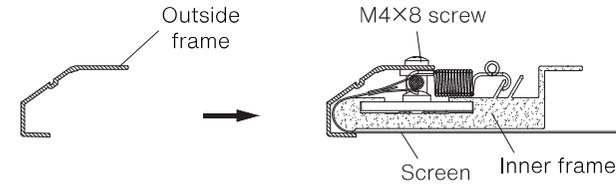
5.2 Adjust the outer frame at the corner to the smallest gap, and then tighten the screws. Lock the corners one by one according to this method, and finally deal with the splicing of the horizontal outer frame (if the gap is found to be too large, you can push the left and right outer frames inward)
