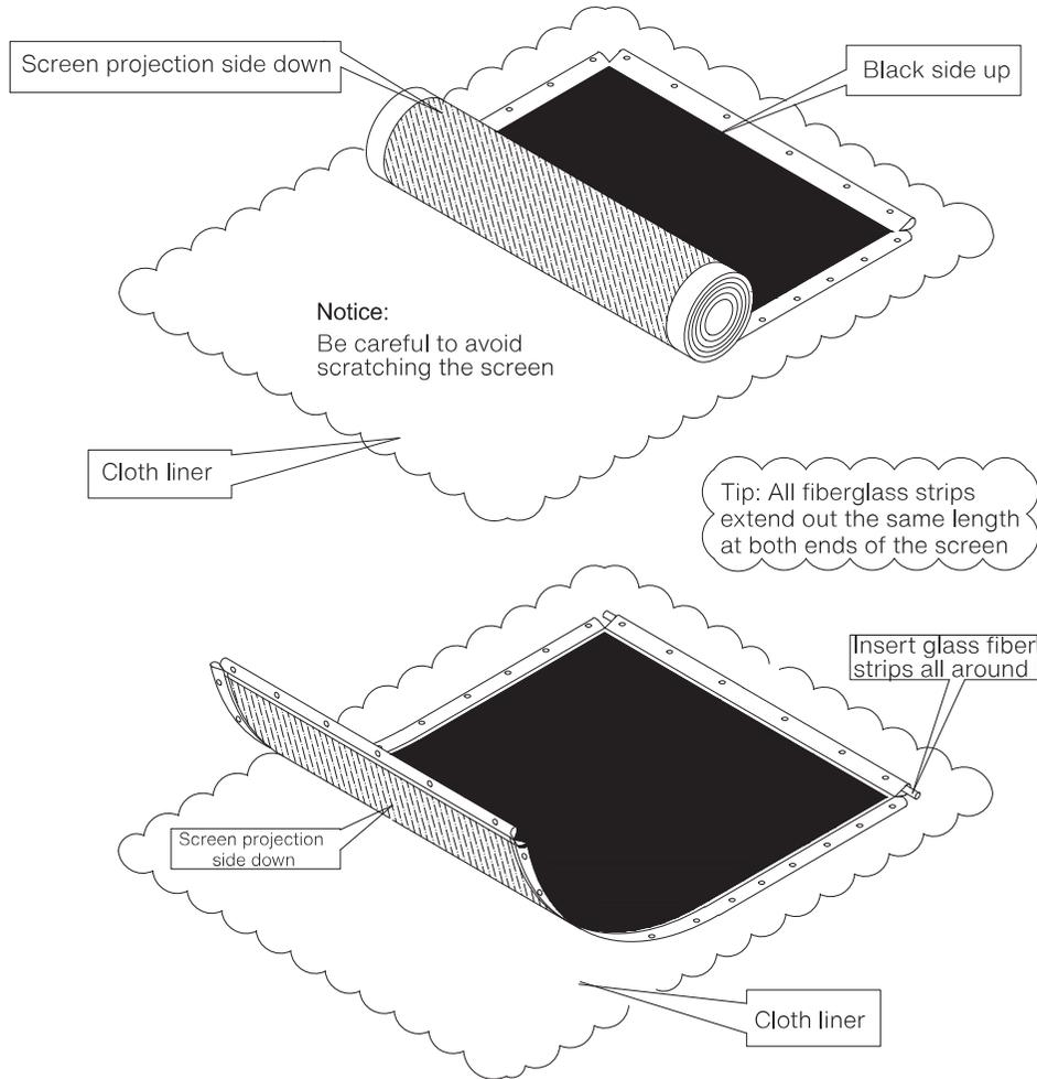
4.3 Place the assembled border on the screen. Note: The ultra-short focus anti-light screen has an up-and-down direction (other curtains have no direction). If it is an anti-light screen, it should be matched with the direction of the frame. Adjust the position of the screen according to the lines marked on the four corners of the screen.
