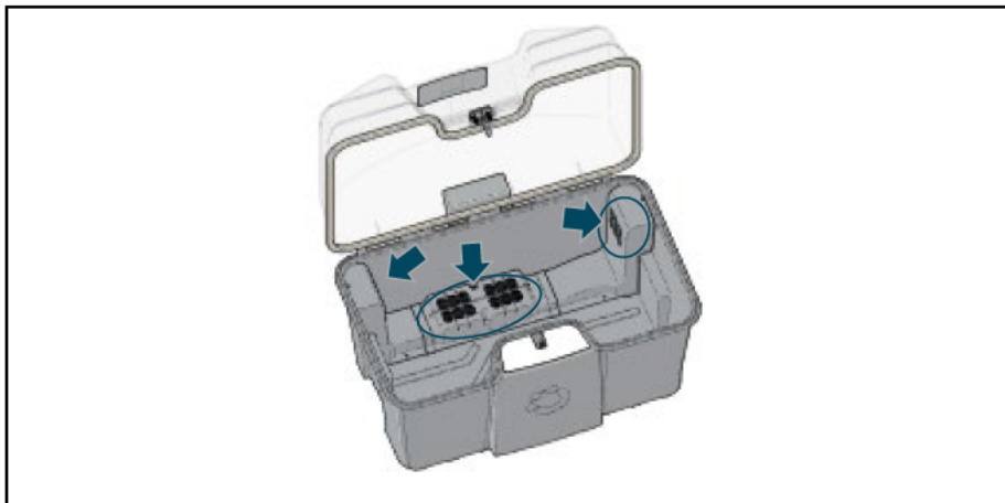
Figure 22 Keep these areas free of dust and debris to maintain cycle efficiency
