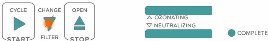
Figure 7 Filter LED is lit to indicate either the filter is approaching the end of its useful life (slow flash) or that the filter must be replaced (solid, not flashing).
