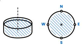
\*Do Not Skip This Step. This is where 90% of installation mistakes occur.\* Once the liner is centered, you will need to temporarily attach 4 points of the liner to the pool wall (North, South, East, West). This will ensure your liner is perfectly even all the way around. If you only start with one point and start attaching the liner by working your way around the pool, the liner will not be straight and may seem short or too small for the pool.
