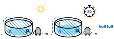
As the vac runs, and the liner is adjusted to your likeness, you can start filling the pool with water. You think your work is done, but it is not done yet. Fill during hot and sunny hours only. Fill only when someone is home to check on the filling process every 20 minutes until the pool is half way full. If something loosens, pulls inwards, or slips at the top, turn everything off, adjust, tighten clamp down, and resume filling.
