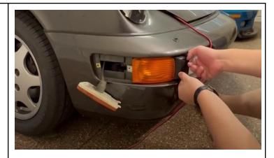
d) Now remove the plastic part in order to access the Parking Light housing.
