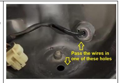
b) Pass the wires to the connector.
