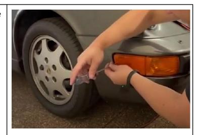
b) To remove the second screw partially retaining the Parking light housing.
