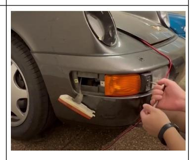
e) You can now access the connector of the Parking Light housing in order to plug the wires from the LED Angel Eye.
