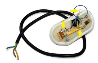
Using the Solder Seal Wire Connector Heat Shrink provided with the kit or other type of connector if you want, connect the wires from the LED Turn Signal directly to the wiring harness using the following color code:
