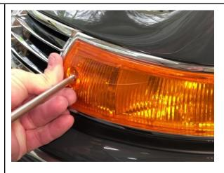
Then, remove the two screws retaining the Turn Signal housing in place.
