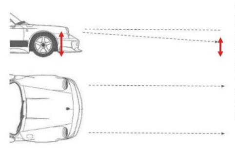
The upper cutoff shadow line with low beams should be 2" lower than the height of the projector from the ground when measured 25' from the vehicle. This measurement is easily taken with the vehicle parked 25' from a wall, measuring the cutoff line on the wall.
