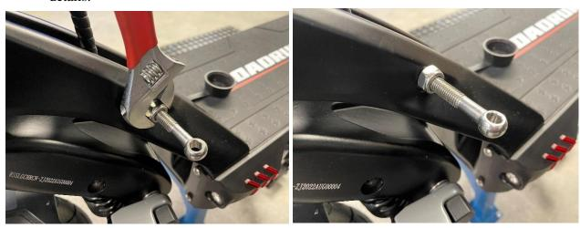
6.) Take the shorter eye bolt and attach the nut to the end. Tighten it down so the nut is about halfway down the threads:
