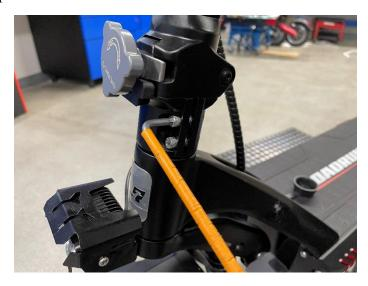
2.) Then, place the mounting bracket onto the folding base, and attach the two bolts we just removed. Tighten down all the way:
