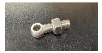
7.) Use your fingers to thread the eye bolt onto the mounting bracket. You may need to use the adjustable spanner to thread the nut far enough onto the bracket. Once the nut is touching the mounting bracket, use the adjustable spanner to tighten down the nut.
