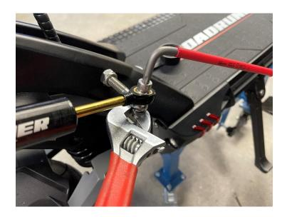
12.) The last step is to adjust the collar along the damper so that the steering will turn in both directions. To do this, turn the handlebars so that they are at dead center (pointed straight). Then, slide the damper into a position where the gold rod on either side of the damper cylinder are equal:
