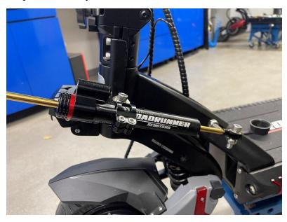
11.) Attach both 8mm nuts to the bottom of the M8 bolts we just attached. Tighten using the adjustable spanner and the 6mm allen as a counter torque:
