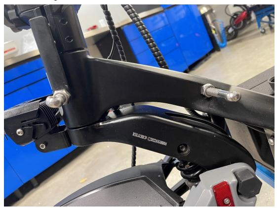
9.) Take the damper and slide the collar on. Keep the two 4mm bolts loose for now.
