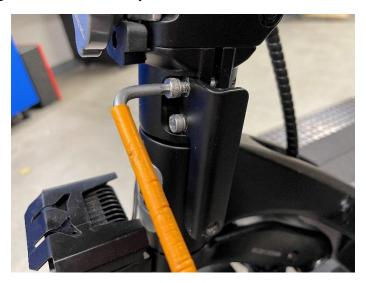
3.) Take the longer eye bolt and begin screwing the 10mm nut onto the end of the eyelet. You will want to screw it down onto the threads until the nut is about halfway through the threads, like so:
