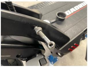
5.) Take the adjustable spanner and tighten down the nut until snug. You will want the eyelet to be slightly diagonal, as you will want it to align with the other eyelet. See step 8 for details.
