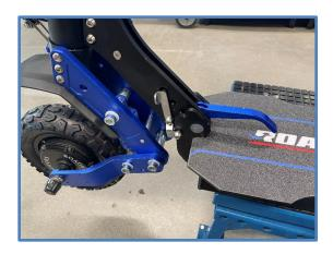
1. Begin by moving the safety lever into its lowered position.
