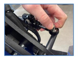
7. Now slide the clamp onto the steering damper. Don't tighten the clamp down just yet. The damper is oriented in the below photo exactly how we want it on the scooter (lefthand side is the front, righthand side is the rear)
