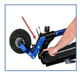
Press the silver snap back towards deck of scooter to completely remove the black post from the upper slot.
