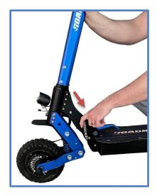
Pull the blue safety lever down to the deck. Press the silver snap back so that the stem completely folds down as shown in picture.
