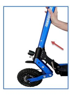
Keep pressing the silver snap and push the stem vertical to ground.
