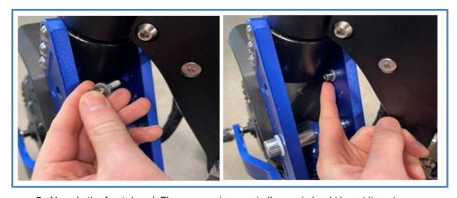
5. Now do the front dowel. The process is very similar, and should be a bit easier. Start by placing the washer onto the M5 bolt, and place it through the hole on the righthand side of the blue arm. Then hand tighten the dowel onto the other end of the M5 bolt. **Remember:** do not tighten all the way yet.
