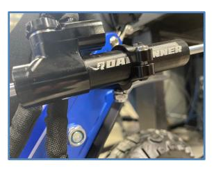
10. Place the M8 spring washer onto the underside of the M8 bolt, then start threading the M8 locking nut onto the bolt (following the spring washer).
