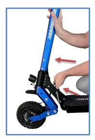
After the stem is locked in an upright position, push the stem forward to remove pressure from the safety lever while simultaneously pushing the blue safety lever with opposite hand up towards the stem until lever is locked in place.
