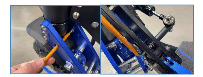
14. Finally, use the 5mm allen to tighten down the two M5 bolts. This is the last step. Please contact RoadRunner Scooters if you have any questions!
