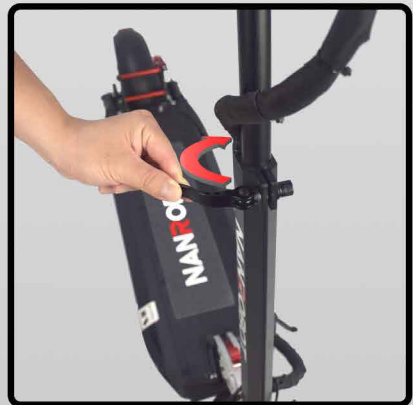
④ Tighten the fastening buckle and turn it back in the direction of the arrow.
