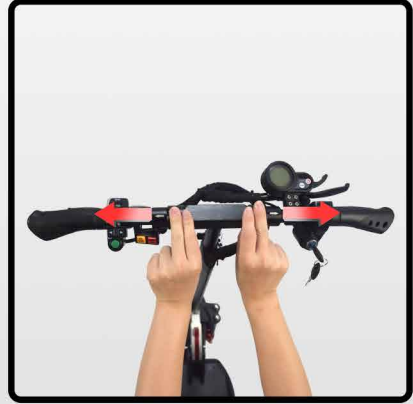
② Push the folding sleeve in the direction of the arrow
