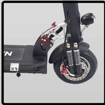
④ When the silver post is caught in the upper slot, the unfolding is completed
