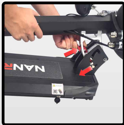
② Keep pressing the red folding button so that the silver post completely leave the lower slot
