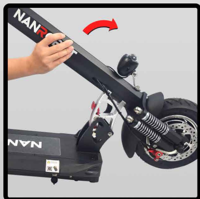
③ Push back the pole in the direction of the arrow
