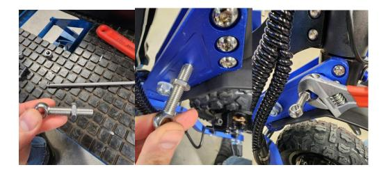
5. Now we will slide the clamp onto the steering damper. Don't tighten the clamp down just yet. The damper is oriented in the below photo exactly how we want it on the scooter (lefthand side is the front, righthand side is the rear)
