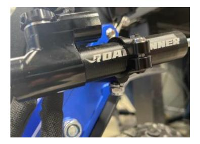
9. Use the 13mm socket (or adjustable spanner) to tighten the bolt onto the underside of the nut. Repeat this step for both M8 bolts on either eyelet. Use the 6mm allen as a counter torque.
