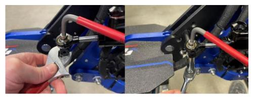
10. Now we will position everything so it is possible to turn the steering equal amounts in either direction. Start by adjusting the damper along the length of the rod so that there is an equal amount of silver rod on either side.
