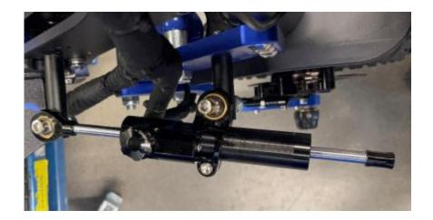
11. Tighten down the 5mm bolt on the clamp using a 5mm allen.
