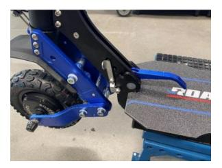
2. Get the longer eyelet bolt and screw in the nut to about 1/3 of the bolt lenght.
