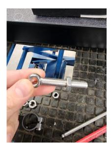
3. Screw it into the frame and tighten the nut with the adjustable spanner wrench.
