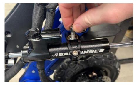
8. Start threading the M8 locking nut onto the bolt.
