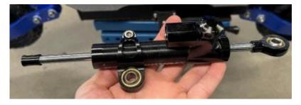
6. Place the eyelet above the rear eyelet bolt hole and start threading the M8 bolt through the eyelet in the damper into the eyelet of the bolt. Once you can no longer tighten it with your fingers, use the 6mm allen to tighten down the rest of the way.
