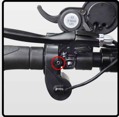
Check whether the voltage lock is locked and fasten as the picture show
