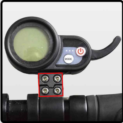
Check whether the LCD control panel is locked and fasten as the picture show
