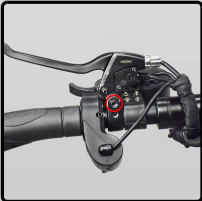
Check whether the brake handlebar is locked and fasten as the picture show
