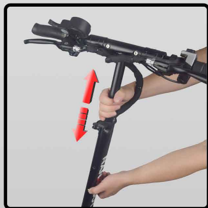
③ Press the silver buckle and adjust the pole up or down as you wish ( there are three heights to choose from )
