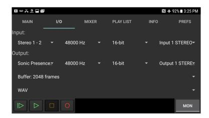
Here you can select the Input and Output sample rate and the word size of 16 or 24 bits. The larger the word size, the higher the audio quality. At the very bottom of the screen, you select the file type. You can choose between an uncompressed WAV file or various compressed file formats.
