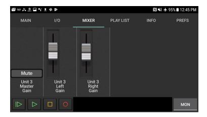
The sliders labeled Unit 3 control the Mic Volume for the Left and Right channels. Since there are no calibration marks, getting a balance between the channels for stereo can be a bit tricky. The Mute button shuts off the audio. The MON button routes the Input signal to the Output for monitoring.
