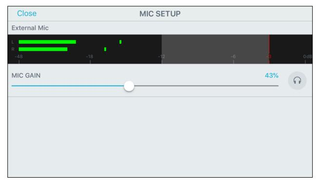
You see "External Mic." Indicated at the top and the large audio level meters. Below the meters is the Input level control. It should initially be set to 50%, which is the calibrated level of the SP15C. That level is set so that 0dB on the meter scale is equal to a level of 120dB SPL.
