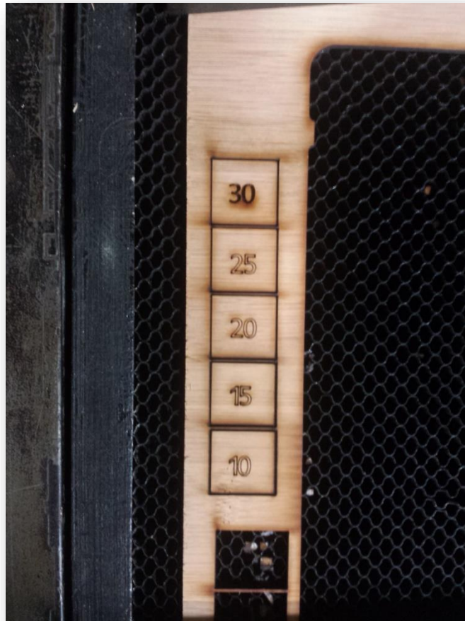
Test cuts in 1/4" maple plywood
