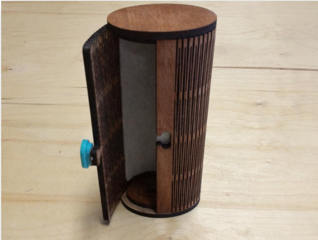
Glasses Case – a 360 degree living hinge
