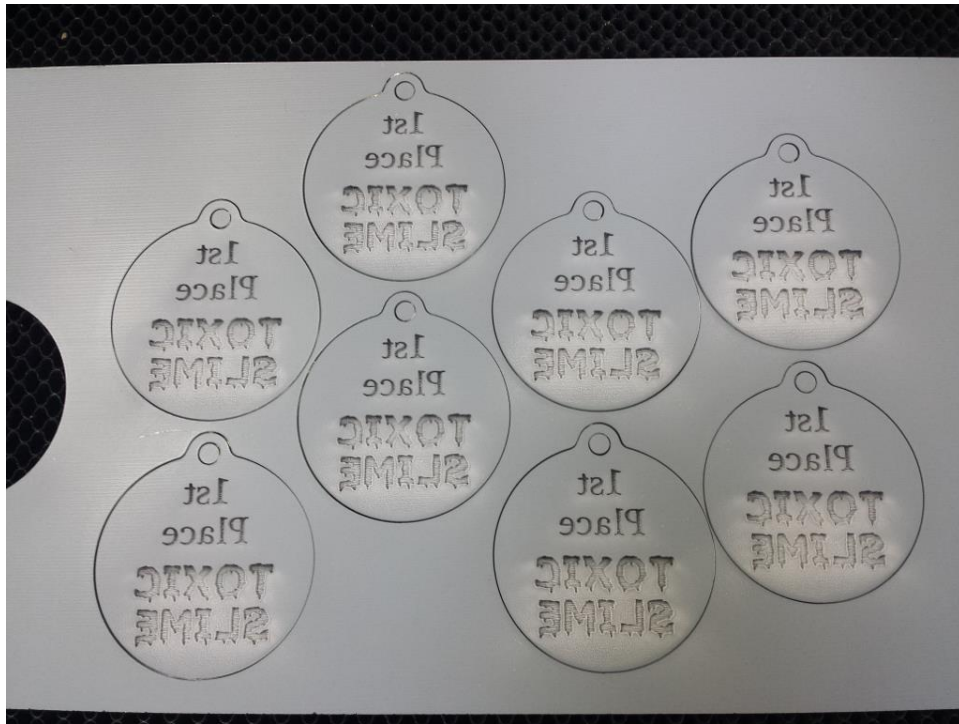
Flipped text engraved from the back
