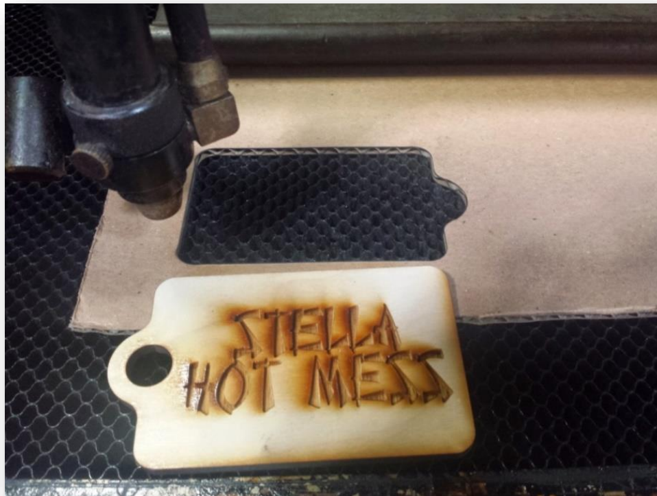
Cardboard Jig in the Laser
