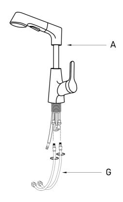
Swivel the hot and cold water pipes (G) into the faucet body (A).
