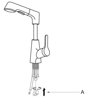
Connect the adapter of the gravity hammer rope to the faucet body.
