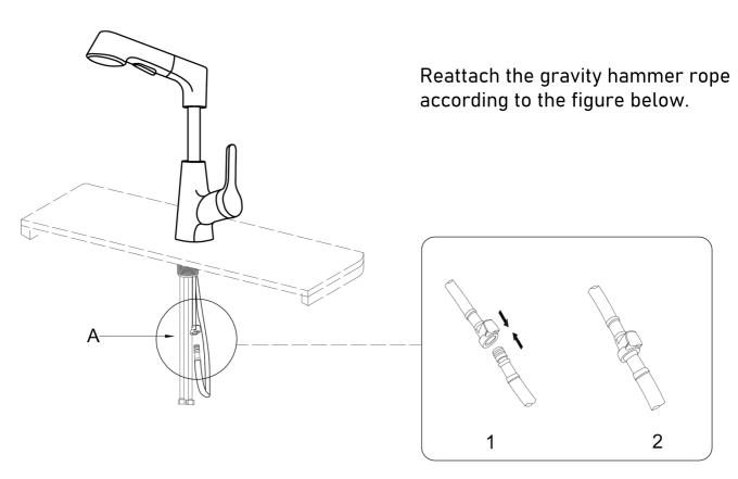
Step 6. Install gravity hammer
