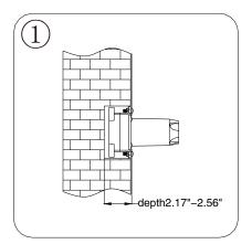
According to the basic size of the embedded box, use a special tool to cut the main hole on the solid wall. The depth of the hole is shown in the figure. The distance between the surface after the final treatment of the wall and the bottom surface of the hole should be considered between 2.17"-2.56".
