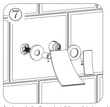
As shown in the figure, install the outlet pipe and wind the sealing tape counterclockwise at the thread connection. It is required to wrap several rounds to ensure the sealing effect.
