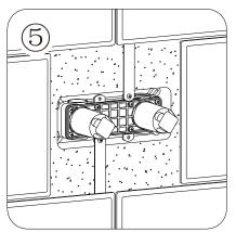
Once again, make sure that the pipe connection is correct and there is no leakage in the water test. After the installation of other embedded components of the shower, seal and fix the embedded box and pipe with packing. At this point, the solid wall embedded box is installed and the plastic protective cover is taken out.
