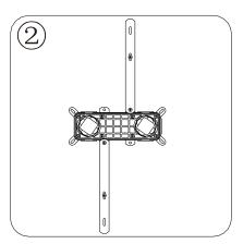
First find a good stainless steel fixing bracket, with screws locked in the embedded box protruding position.
