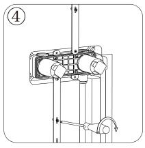
Open the water source to test whether the left and right inlet pipes are tightly connected without leakage. After the inlet pipes are tested and closed, adjust the flow switch to be in the open state to test whether the mixed outlet pipes are tightly connected without leakage. At the same time the function of water retention, according to the embedded box is installed into the solid wall inside the tapping screw embedded box is fixed on the wall.
