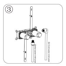
As shown in the figure, pre-bury the intake water pipe, pay attention to the upper and lower direction of the embedded box, the lower right interface is connected with the hot water pipe, the right interface is connected with the cold water pipe.
