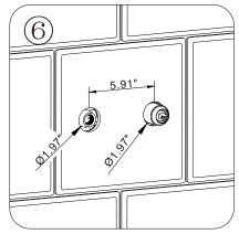
As shown in the picture, paste the ceramic tile, and open two holes with a diameter of 1.97" in the middle, and the distance between the two holes is 5.91".
