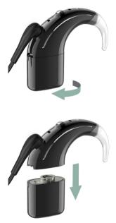
1. Twist the battery module as shown to release it from the processing unit.
