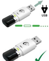
4. The LED changes to steady green when the module is fully charged.
