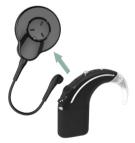
2. Lift the microphone cover from the bottom edge, then lift it up to remove.
