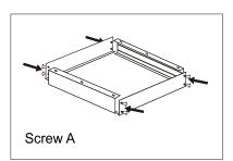
Assemble the four sides with 2 X screw A each to create the frame.
