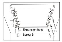
Fix the frame to the ceiling with screw B and expansion bolts.
