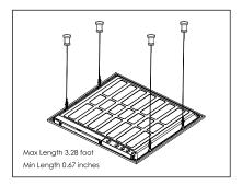
Release wire and connect to panel light. Buckle up the suspension hooks to the triangle hooks attached on panel light.
