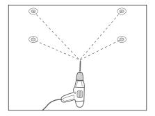
According to the length and the width of the panel light, drill four mounting holes on the mounting position.
