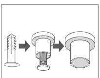
Use self-tapping screw to lock the upper cover to mounting hole.
