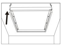
Once securely mounted to the ceiling disassemble one end (without mounting screws to the ceiling).
