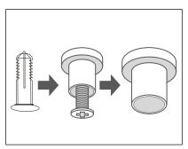
Use self-tapping screw to lock the upper cover to mounting
