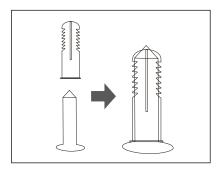
Fix the screw inside the expansion bolt to get the self-tapping screw.
