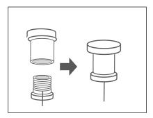
Twist matching the lower cover to the upper cover. Complete the connection of cable and bearing load.
