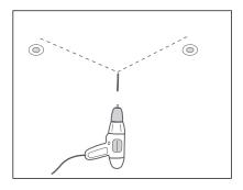
According to the length and the width of the panel light, drill four mounting holes on the mounting position.
