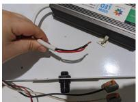
Once the wires have been disconnected from the driver, remove the driver from the mirror housing. (Figures a. and b.)
