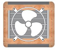
**Wide Mount:** The AFG can be mounted on a wide louver, but additional mounting steps must be taken in order for the fan to work properly. As shown in Figure 2.1B, two additional boards must be fastened to the boards framing the gable vent so the AFG can be mounted securely.
