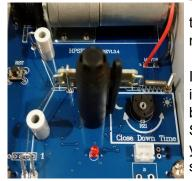
cover the controller with the box. Wait 5 seconds. The door should start lowering. Once it reaches the bottom, you can remove the cover and it will return to the top. Set-up is now complete.
