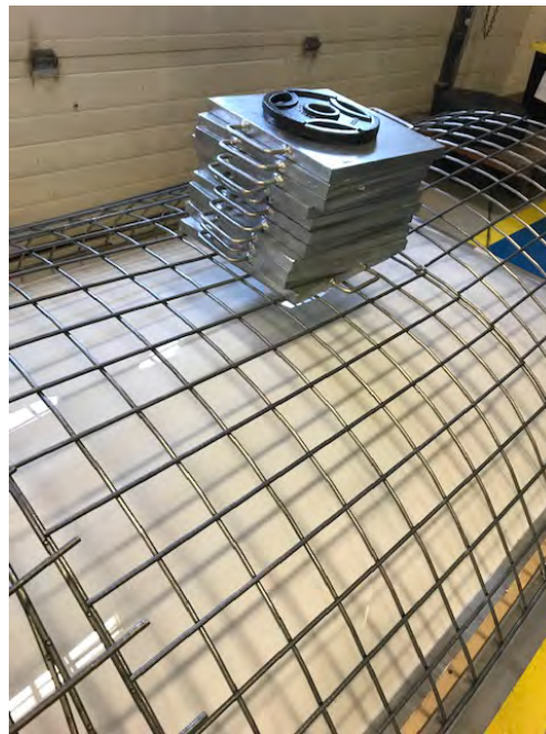
Photo 4. - Test weight (622lb) front end of STS Skylight
