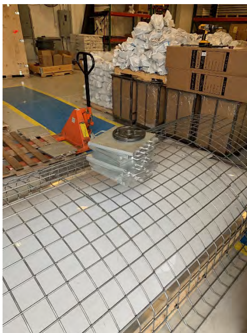
Photo 4. - Test weight (622lb) front end of SRS Skylight
